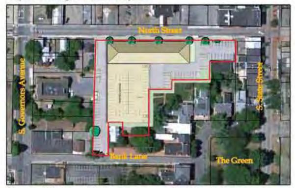
Conceptual Multi-Level Parking Structure and Mixed-Use Building Proposed Parking Provided - 55 Surface Spaces & 65+/- Spaces per parking structure level
